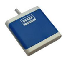
The Omnikey 5022 CL from HID is a 13.56 MHz contactless smartcard reader that supports a broad range of contactless credentials including iClass, MIFARE, MIFARE DESFire and Seos. Providing Windows Plug-and-Play support, this reader can be seamlessly integrated into most end-user environments with little to no administration.
